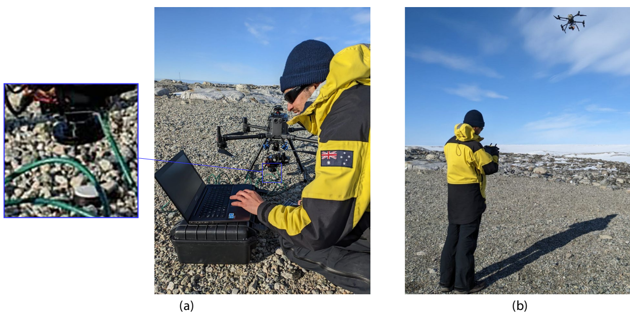
Fig. 10. Aerial hyperspectral data collection setup in ASPA 135. (a) Ground setup for white reference (WR) calibration using the Nano-Hyperspec camera mounted on the DJI M300 RTK. The hyperspectral camera is directed at a Spectralon panel on the ground to calibrate exposure settings prior to UAV flights. (b) DJI M300 RTK equipped with the Nano-Hyperspec camera conducting flight operations over ASPA 135.
