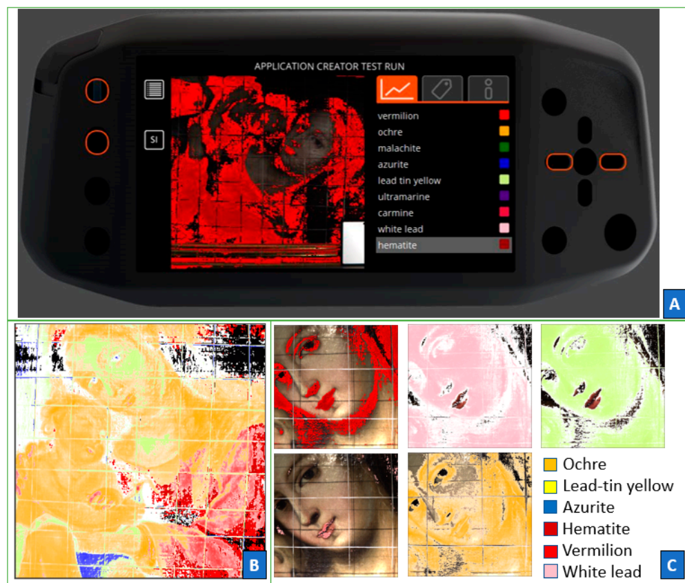
Figure 8. Application of the classification method for the handheld VNIR hyperspectral camera using
